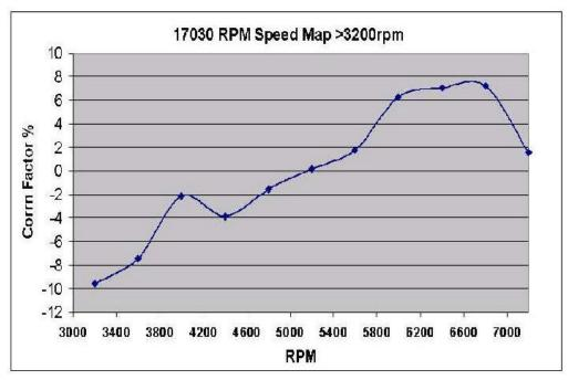
Being a speed density system it is no surprise then that the next fuel map is an engine 'speed' map. This is a map that gets navigated with respect to engine rpm. The higher the rpm, the further along the map the ECU goes. There are two speed maps, one for below 3200rpm and one for above 3200rpm. These maps are twinned with the two density map curves above. This rpm correction map is a little more
