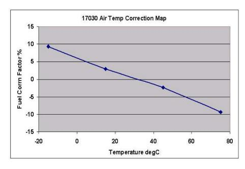
As mentioned earlier, intake air temperature affects the air mass for a given volume so the ECU needs to correct the fuelling still further. This is the next map in the series to get consulted by the ECU. The cooler the air the more dense the air is so the more fuel should be added. According to theory this map should be a straight line and it is! I was expecting a slightly steeper slope to the line in theory BTW. I may have to recheck my air temperature sensor calibration.
