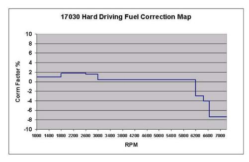
At high load AND rpm well above idle the ECU then consults an extra rpm correction map. On the mk1a this has mapping points at 1800, 2600, 3000, 6200, 6450, 6650 and >6650 rpm. This odd looking map is shown. This provides tighter control of the fuelling when driving the car really hard. As you can see it actually reduces the fuelling above 6200rpm. You can also see how crude this correction map is as it does not interpolate between map
