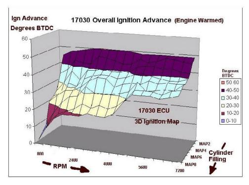
injectors to protect the catalytic converter from any unburnt fuel. As the UK mk1 MR2 does not have a cat, this function seems obsolete but it is still there in the ROM code and it does cut the fuel if no spark occurs (it actually waits until there are several failed sparks before cutting the fuel). Here is a 3D graph showing the ignition advance in degrees BTDC for the 89661-17030 ECU assuming the following conditions: Engine is fully warm, car is being 'driven' i.e. throttle being pressed.
