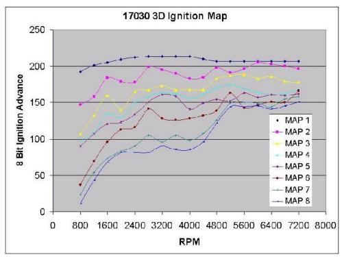
the profile used when the car is being driven hard and cylinder filling is at the highest. See how the ignition timing tends to advance with increasing rpm and how it retards for the higher MAP sensor curves where cylinder filling is good.
