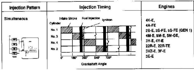
Some readers may initially dispute the simultaneous injection claim as the electrical wiring shows the 4 injectors wired in pairs. The ECU has two outputs feeding each pair hinting at a grouped injection system. Sadly those two outputs are actually strapped together inside the ECU! There is only one driver transistor inside the ECU to control all 4 injectors in parallel. I'm afraid it really is a simultaneous system. I think some Jap and US mk1 variants have grouped injection.
