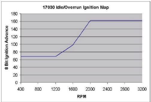
The ECU uses this basic ignition map whenever the car is being 'driven', i.e. when the throttle is being pressed. If the driver lifts off the throttle then the car reverts to a much smaller idle ignition map. This crude map only has 3 rpm sites at 1200, 1600 and 2000rpm. It is unaffected by cylinder filling. If the car is at high rpm when the throttle is lifted off (overrun) then the ECU uses the value in the 2000rpm site. As the fuel is cut off during overrun
