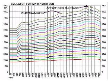
The PC ECU emulator shows the fuelling as a series of curves. Each point on each curve represents a complete fuelling calculation running the same code as the ECU. The emulator includes all the fuel maps and corrections and assumes a fully warm engine with medium to high throttle and 27degC air temperature.
