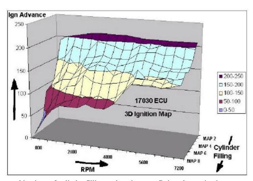
other words, the ECU can skate anywhere on the colored surface, not just on the gridlines) You can clearly see how technically advanced this system is compared to the mechanical advance/retard mechanisms in older vehicles. The engine tuner has complete control over the shape of this 3D map and can alter any section of it by changing a few values in the 3D table. This allows precise control to find the optimum setting for the ignition timing across all
