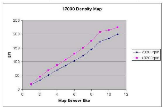
This is a simple 2D graph of MAP sensor vs. fuel duty. This map should be a straight sloping line according to the Universal Gas Law. As you can see from the graph below it IS (nearly) a straight line! The bump in the line close to maximum MAP sensor levels would cause a slight degree of over fuelling at high load, probably
